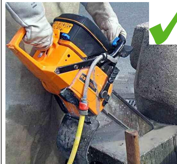
Concrete cutter fitted with a hose to enable Effective dust suppression.
