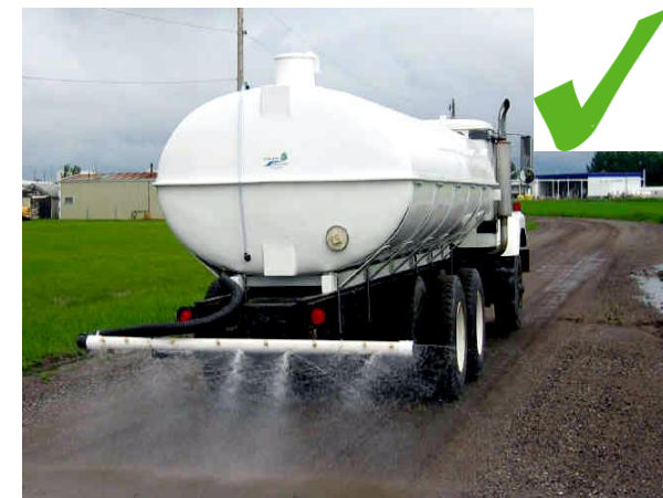
Water-truck in use to keep trafficked routes Wet down to aid dust suppression.
